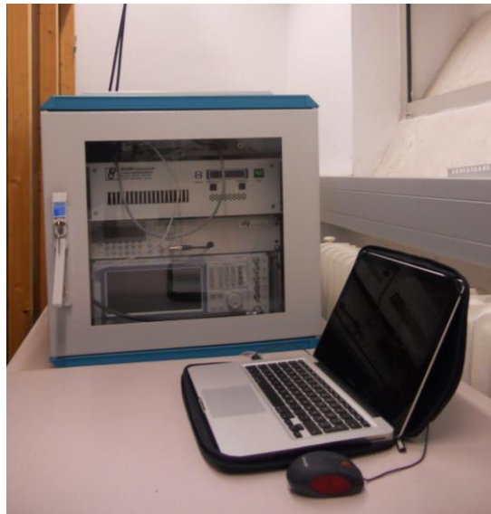
Figure 3.3: Signal generating hardware, amplifier and power meter, built in a 19" rack (background) and laptop computer with control and recording software (foreground), installed at the Institut für Umwelthygiene, Kinderspitalgasse, 1090 Vienna
